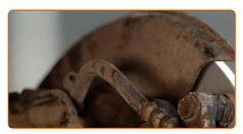
Clean dirt from the brake hose bolt. Use a wire brush. Use a brake cleaner.
