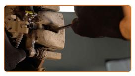
Remove the brake caliper. Use a crowbar.
