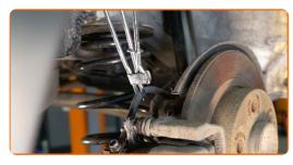
Unscrew the brake hose from the brake caliper. Use a combination spanner #11.
