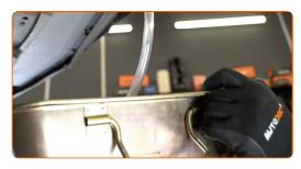
Open the coolant drain tap. Use a flat screwdriver.
