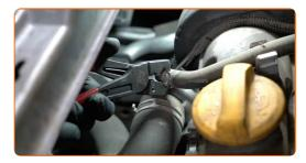
Detach the coolant hose. Use a flat screwdriver.
