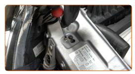
Remove the air distribution housing assembly.
