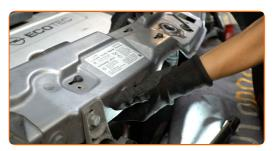
Screw in the fasteners of the air distribution housing assembly. Use Torx T20.
