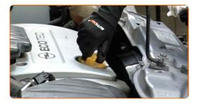
Tighten the oil filler cap.
