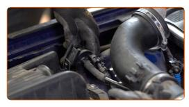
Take off the filter lid. Remove the filter element from the filter housing.
