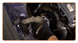
Replacement: engine mounts – VAUXHALL Astra Mk IV (G) CC (T98). Tip:
