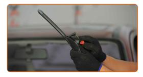
Remove the blade from the wiper arm.
