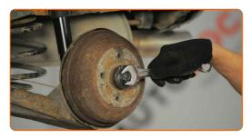
9 Remove the brake drum.
