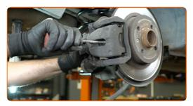
10 Remove the brake caliper.
