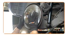
Tighten the brake disc fastening. Use Torx T30. Use a torque wrench. Tighten it to 8 nm torque.
