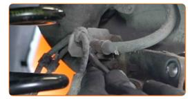
Detach the ABS sensor connector. Use a crowbar.
