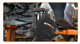
Install the brake caliper and fix it. Use a drive socket #13. Use a combination spanner #17. Use a torque wrench. Tighten it to 25 nm torque.
