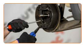
Take out brake pad retainer springs from the holes. Use pliers.
