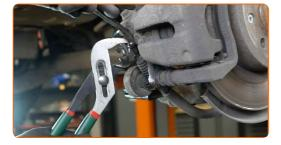
Unscrew the brake caliper fastening. Use a combination spanner #13. Use a combination spanner #17.
