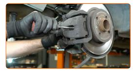
10 Remove the brake caliper.
