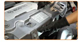
Screw in the fasteners of the air distribution housing assembly. Use Torx T20.
