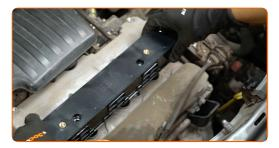
Tighten the ignition coil bolts. Use Torx T30. Use a torque wrench. Tighten it to 7 nm torque.
