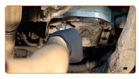
10 Remove the transmission fluid pan.
