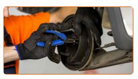
15 Remove the brake pads.
