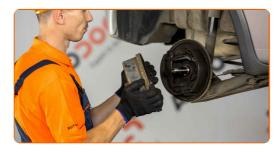
Disconnect the parking brake cable from the parking brake lever. Use round-nose pliers. Use a flat screwdriver.
