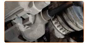
Tighten the fastener connecting the ball joint to the steering knuckle. Use a combination spanner #18. Use a drive socket #18. Use a torque wrench. Tighten it to 30 Nm torque.
