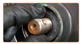
Screw the nut of the drive shaft. Use a drive socket #30. Use a ratchet wrench.
