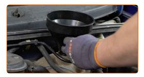
Pour coolant in the coolant reservoir.
