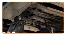
27 Remove the hydraulic transmission jack.
