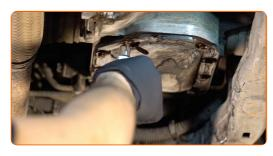
10 Remove the transmission fluid pan.
