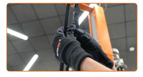
Remove the blade from the wiper arm.
