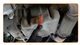
Unscrew the drain plug. Use Torx T40. Use a ratchet wrench.
