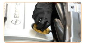
Tighten the oil filler cap.
