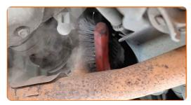
Detach the oxygen sensor connector.
