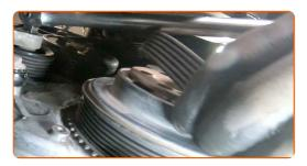
9 Return the tensioner pulley to its initial position.
