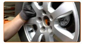
Unscrew the wheel arch cover fasteners. Move the part aside. Use Torx T30. Use a ratchet wrench.
