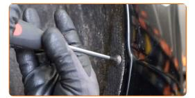
Pull aside the V-ribbed belt tensioner pulley. Use a 1/2" square drive extension bar.
