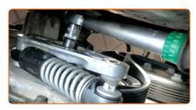
Pull aside the V-ribbed belt tensioner pulley. Use a 1/2" square drive extension bar.
