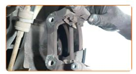
Clean the brake disc fastener. Use a wire brush. Use WD-40 spray.
