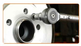
Clean the brake caliper bracket of dirt and dust. Use a wire brush. Use a brake cleaner.
