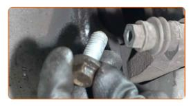
Remove the brake caliper bracket.
