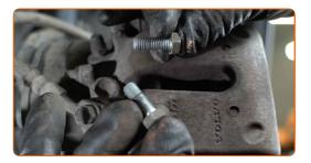
Remove the brake caliper.
