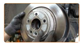
Clean the wheel hub fasteners. Use a wire brush. Use WD-40 spray.
