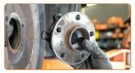
Remove the brake disc cover.
