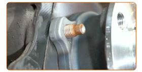
Tighten the wheel hub fasteners. Use Torx T55. Use a torque wrench. Tighten it to 110 Nm torque.
