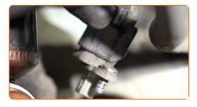
Remove the fastening bolt.
