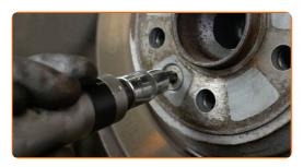
17 Remove the fastening bolt.
