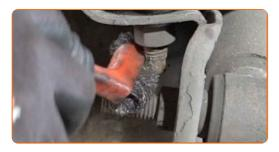
Unscrew the lower fasteners of the shock absorber. Use a drive socket #18. Use a ratchet wrench.
