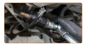
Tighten the shock absorber mount fasteners. Use a drive socket #10. Use a torque wrench. Tighten it to 30 Nm torque.
