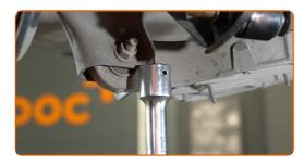
Tighten the lower fastener of the shock absorber. Use a drive socket #18. Use a torque wrench. Tighten it to 150 Nm torque.
