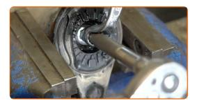
Remove the shock absorber mount, dust boot, and bump stop.
