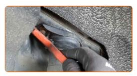
Unscrew the shock absorber mount fasteners. Use a drive socket #10. Use a ratchet wrench.
