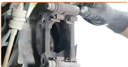
**18** Clean the brake disc fastener. Use a wire brush. Use WD-40 spray.
