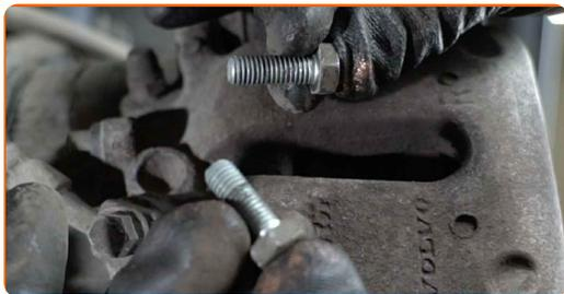
**12** Remove the brake caliper.
