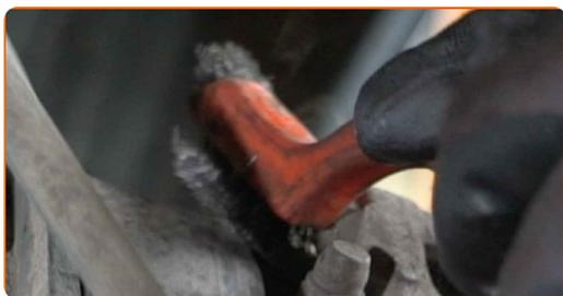
**10** Unscrew the brake caliper fasteners. Use a combination spanner #15. Use a drive socket #13. Use a ratchet wrench.
