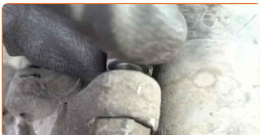
**37** Tighten the brake caliper fasteners. Use a combination spanner #15. Use a drive socket #13. Use a torque wrench. Tighten it to 35 Nm torque.
