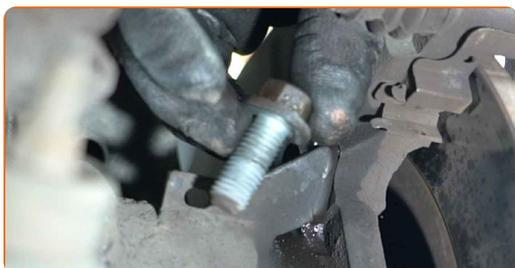
**17** Remove the brake caliper bracket.
