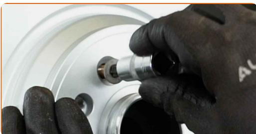
**26** Tighten the brake disc fasteners. Use Torx T50. Use a torque wrench. Tighten it to 15 Nm torque.
