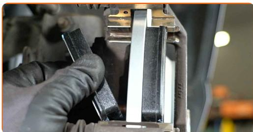
**35** Install the brake caliper and fasten it.
