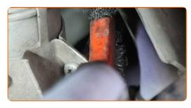
6 Loosen the fuel filter fasteners. Use Torx T30. Use a ratchet wrench.
