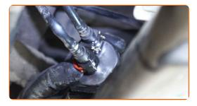
Screw in the fuel filter mounting bracket. Use Torx T30. Use a ratchet wrench.
