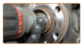
Remove the fastening bolt.
