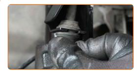
Tighten the lower fasteners of the suspension strut. Use a drive socket #15. Use a torque wrench. Tighten it to 110 Nm torque.
