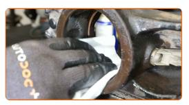
Install the new wheel hub together with the bearing. Use a bush and bearing driver set. Use a bearing separator.
