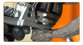
Detach the driveshaft from the steering knuckle.
