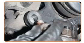
Screw in the fasteners of the brake caliper bracket. Use a drive socket #18. Use a ratchet wrench.
