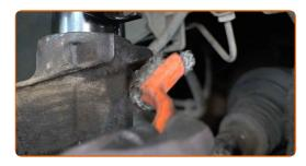
Unscrew the lower fastener connecting the shock strut to the steering knuckle. Use a drive socket #15. Use a ratchet wrench.
