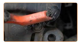
Unscrew the fasteners of the brake disc cover. Use a drive socket #8. Use a ratchet wrench.
