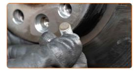
18 Remove the brake disc.
