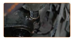
Remove the fastening bolt.
