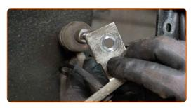
Clean the fastener connecting the tie rod end to the steering knuckle. Use a wire brush. Use WD-40 spray.
