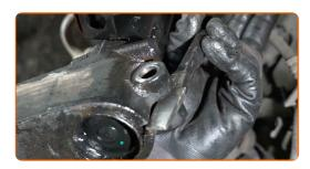
Disconnect the steering knuckle from the suspension strut. Use a rubber mallet.
