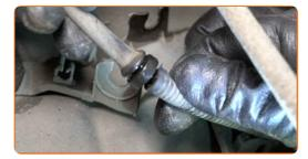
Unscrew the fastener connecting the stabilizer link to the shock strut. Use a drive socket #15. Use a ratchet wrench.
