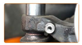
Reconnect the sway bar link to the suspension strut.
