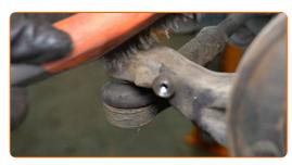
Unscrew the fastening nut connecting the tie rod end to the steering knuckle. Use a drive socket #22. Use a ratchet wrench.
