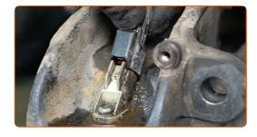
Disconnect the ABS sensor wiring.
