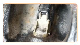
69 Install the brake disc cover.
