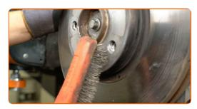
Unscrew the brake disc fasteners. Use Torx T50. Use an impact screwdriver. Use a hammer.
