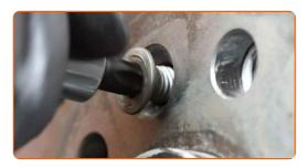
75 Tighten the brake disc fasteners. Use Torx T50. Use a torque wrench. Tighten it to 15 Nm torque.
