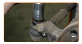
Disconnect the tie rod end from the steering knuckle. Use a ball joint puller.
