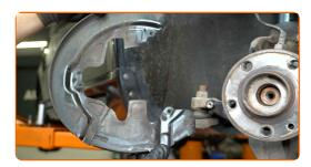
Clean the ABS sensor connector. Use a nylon cleaning brush. Use all-purpose cleaning spray.
