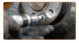
17 Remove the fastening bolt.
