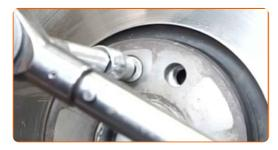
76 Install the brake caliper together with its bracket.
