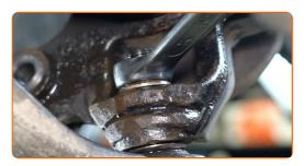
Disconnect the ball joint from the steering knuckle. Use a ball joint puller. Use a crowbar.
