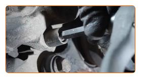
Remove the brake caliper.
