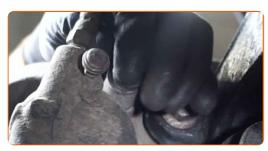
Install the brake pad retaining clip.
