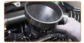
Pour oil into the engine through the filler. Required amount of oil: 5,9 l.
