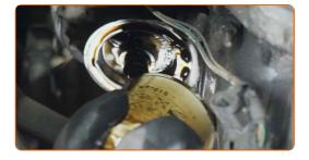
Clean the oil filter seat. Use all-purpose cleaning spray.
