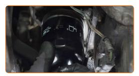
Tighten the oil filter. Remember to observe the recommended tightening torque. Use the 76-14F socket. Use a torque wrench. Tighten it to 17 Nm torque.
