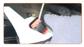
Attach the mass air flow sensor connector.
