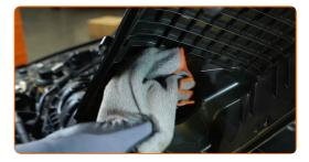
Install the air filter cover. Fasten it.
