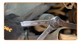
Tighten the tie rod end locknut. Use a combination spanner #19. Use a combination spanner #22. Use a torque wrench. Tighten it to 70 nm torque.
