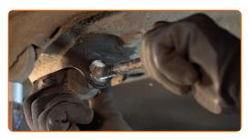
17 Remove the shock absorber. Use a crowbar.
