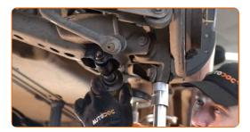
Tighten the top shock absorber fastening. Use a combination spanner #18. Use a drive socket #18. Use locking pliers. Use a torque wrench. Tighten it to 60 Nm torque.
