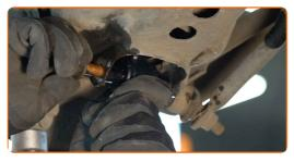
Screw in the lower fastener of the shock absorber. Use a drive socket #18.
