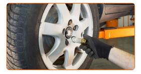
Lower the car and working in a cross order, tighten the wheel bolts. Use wheel impact socket #19. Use a torque wrench. Tighten it to 140 Nm torque.
