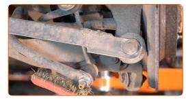
Unscrew the fasteners connecting the stabiliser link to the stabiliser bar. Use a drive socket #18. Use a ratchet wrench.
