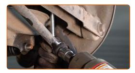
Install the rod fastening to the stabilizer and tighten it. Use a drive socket #18. Use a torque wrench. Tighten it to 60 Nm torque.
