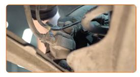
Install the brake caliper retaining spring. Use a rubber mallet. Use a crowbar.
