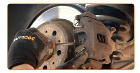
11 Remove the brake caliper.
