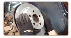
Tighten the brake disc fastening. Use a drive socket #10. Use a torque wrench. Tighten it to 9 Nm torque.
