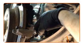
Remove the caliper bracket.
