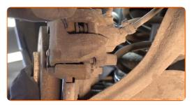
Remove the dust boot caps of the brake caliper guide pins. Use a crowbar.
