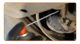
Unscrew the oil filter. Use the 86/14-F socket.
