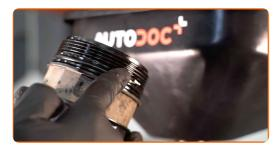
Screw the new filter into its place. Use the 86/14-F socket. Use a torque wrench. Tighten it to 25 nm torque.
