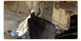
Screw in the new drainage plug and tighten it. Use a drive socket #15. Use a torque wrench. Tighten it to 38 nm torque.
