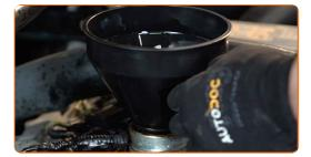
Pour oil into the engine through the filler. Required amount of oil: 4.3 L.
