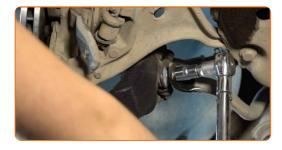
Tighten the fastener connecting the stabilizer link to the shock strut. Use a combination spanner #18. Use a drive socket #18. Use a torque wrench. Tighten it to 50 Nm torque.
