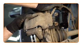
Install the dust boot caps of the brake caliper guide pins.
