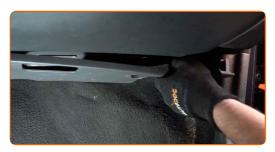
Unscrew the fasteners of the cabin filter housing cover. Use Torx T20. Use a ratchet wrench.
