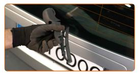
Remove the blade from the wiper arm.
