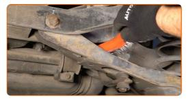
Unscrew the stabilizer rod fasteners. Use a drive socket #16. Use a combination spanner #15.
