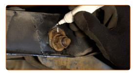
Unscrew the fastener connecting the control arm to the rear subframe. Use a combination spanner #18. Use a combination spanner #19. Use a drive socket #18. Use a ratchet wrench.
