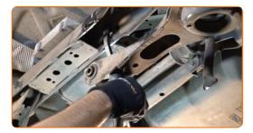
Install the fastening bolt. Use a hammer. Use a crowbar.
