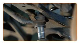
Tighten the fastener connecting the stabilizer link to the stabilizer bar. Use a drive socket #15. Use a combination spanner #16. Use a torque wrench. Tighten it to 50 nm torque.
