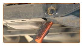
Make a mark on the camber adjustment bolt.
