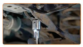
Remove the fastening bolt. Use a pin punch. Use a hammer. Use a crowbar.
