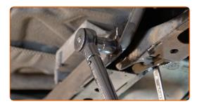
Remove the support from under the arm.
