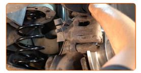
Install the brake caliper retaining spring. Use a rubber mallet.
