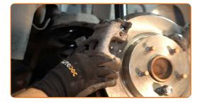
Install the dust boot caps of the brake caliper guide pins.
