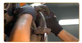
Tighten the brake caliper bracket. Use a drive socket #13. Use a torque wrench. Tighten it to 70 Nm torque.
