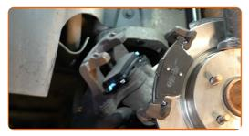
Install the brake caliper and fix it. Use HEX No.H7. Use a torque wrench. Tighten it to 35 Nm torque.
