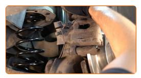
Install the brake caliper retaining spring. Use a rubber mallet.
