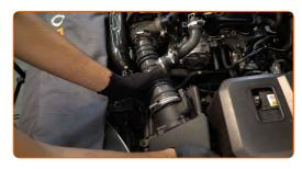
Attach the air inlet pipe to the turbocharger.
