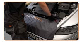
Unscrew the engine cover fastener. Use a drive socket #10.
