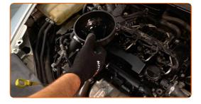
Pour oil into the engine through the filler. Required amount of oil: 4.1 L.
