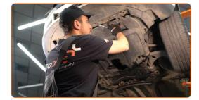
Tighten the fasteners of the oil pan lower cover. Use a drive socket #10. Use a ratchet wrench.
