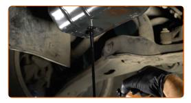
Replacement: engine oil and filter – Volvo V50 MW. Tip:
