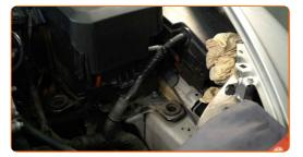
Cover the turbocharger impeller with a microfibre cloth to prevent dirt and foreign objects getting into the system.
