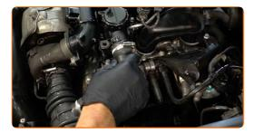
37 Install the clamp of the crankcase ventilation hose.
