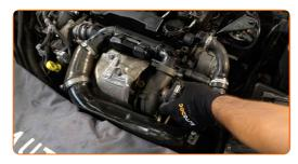
10 Remove the air filter housing retaining spring.
