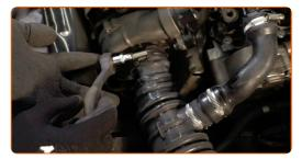
Detach the crankcase ventilation hose clamp.
