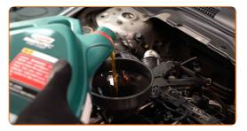
Replacement: engine oil and filter – Volvo V50 MW. Tip from AUTODOC:
