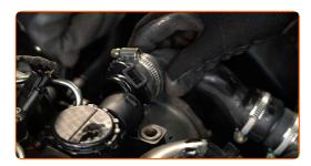
Detach the air inlet pipe from the turbocharger.
