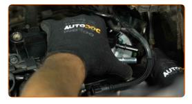
Screw the fixing bolts of the fuel filter bracket. Use a drive socket #8. Use a ratchet wrench.
