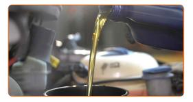
Replacement: engine oil and filter – VW T5 Transporter. Tip from AUTODOC experts:
