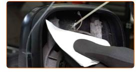
Attach the mirror heating connectors.
