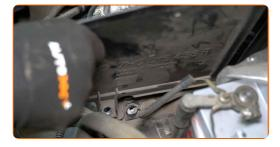
Unscrew the fuel filter bracket. Use a drive socket #10. Use a ratchet wrench.
