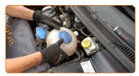
Screw in the coolant reservoir fasteners. Use a Phillips screwdriver.
