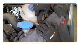
5 Remove the coolant reservoir.
