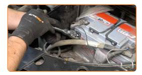
Screw in the fasteners of the back section of the engine cover. Use a flat screwdriver.
