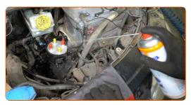
Connect the fuel lines to the new fuel filter.
