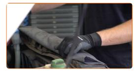
Detach the coolant expansion tank connector.
