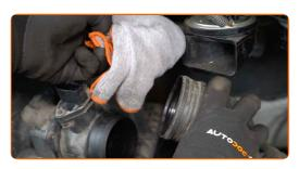
Connect the air intake pipe to the air filter housing.
