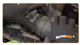
Fasten the clamp on the air intake hose. Use clic-R collar pliers.
