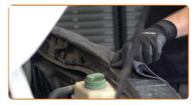
Unplug the mass air flow sensor connector.
