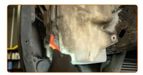
Detach the connector from the windscreen washer pump. Use a mounting lever.
