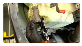
Remove the washer pump seal. Use a mounting lever.
