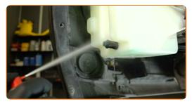
Install a new washer pump seal.
