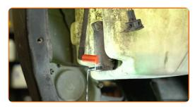
Remove the windscreen washer pump. Use hose removal pliers.
