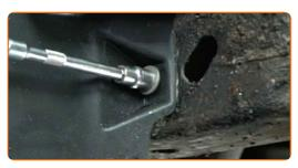
Screw in the fastening bolt of the windscreen washer reservoir's cover. Use a 10 mm socket. Use a ratchet wrench.
