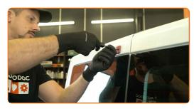
Remove the fastening screws.
