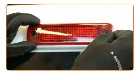
Install the fastening screws.
