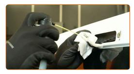
6 Attach the connector to the new brake light.
