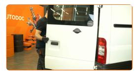
Unscrew the fasteners connecting the rear light to the car body.
