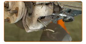
Unscrew the brake caliper fasteners. Use a 13 mm combination spanner.
