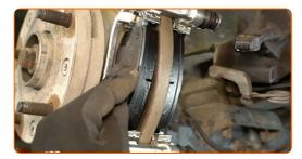
Install the wear sensor on the inner brake pad.
