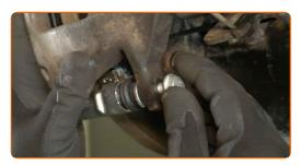
Tighten the fasteners of the brake caliper bracket. Use an 18 mm combination spanner. Use a 13 mm socket. Use a torque wrench. Tightening torque: 31 N·m.
