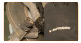
18 Remove the brake caliper bracket.
