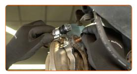
Tighten the fasteners of the brake caliper bracket. Use a 15 mm socket. Use a torque wrench. Tightening torque: 115 N·m.
