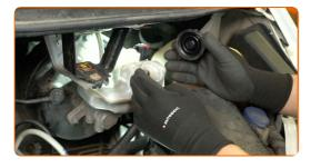
Tighten the brake fluid reservoir cap.
