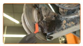
Treat the brake caliper piston. Use a nylon brush. Use a brake cleaner.
