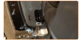
27 Install the brake caliper.
