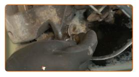
Remove the brake caliper.
