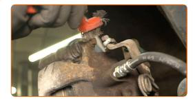
Spread the brake pads apart. Use a mounting lever.
